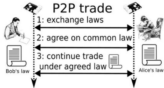
Figure 4: Common law is obtained after a merge process between two laws supplied by each peer. The outcome, when signed by both parties, serve as regulatory basis for the remaining events in the interaction.
