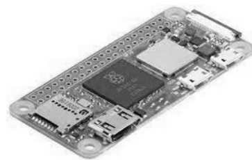
Figure 32: Raspberri Pi Zero is a low power computer. Via de micro USB interface it runs at 5.2V. When connected to WiFi it draws around 200mA which is a total of 1W.
